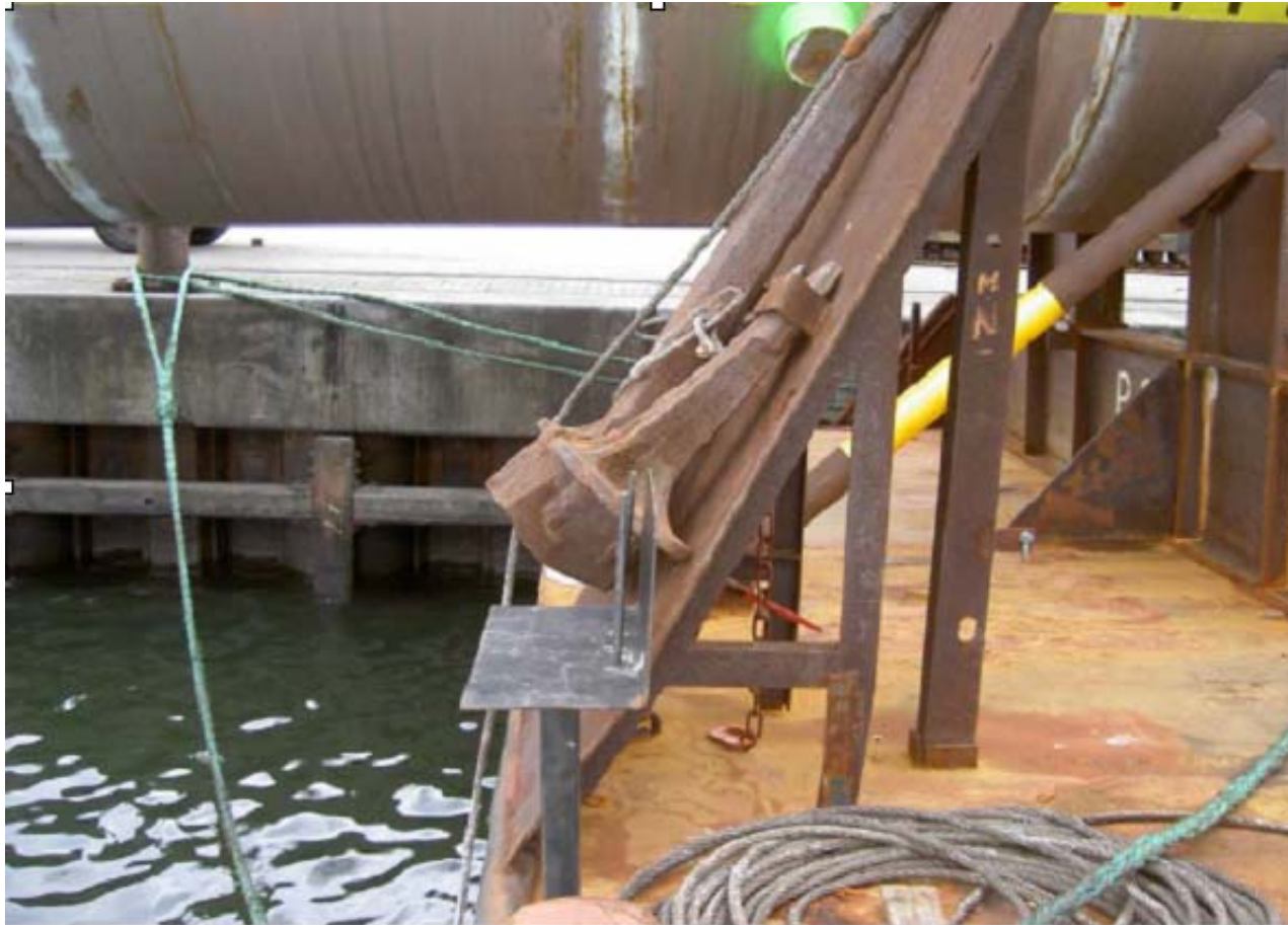
Edge of navigation Light holder extends pass the barge.
