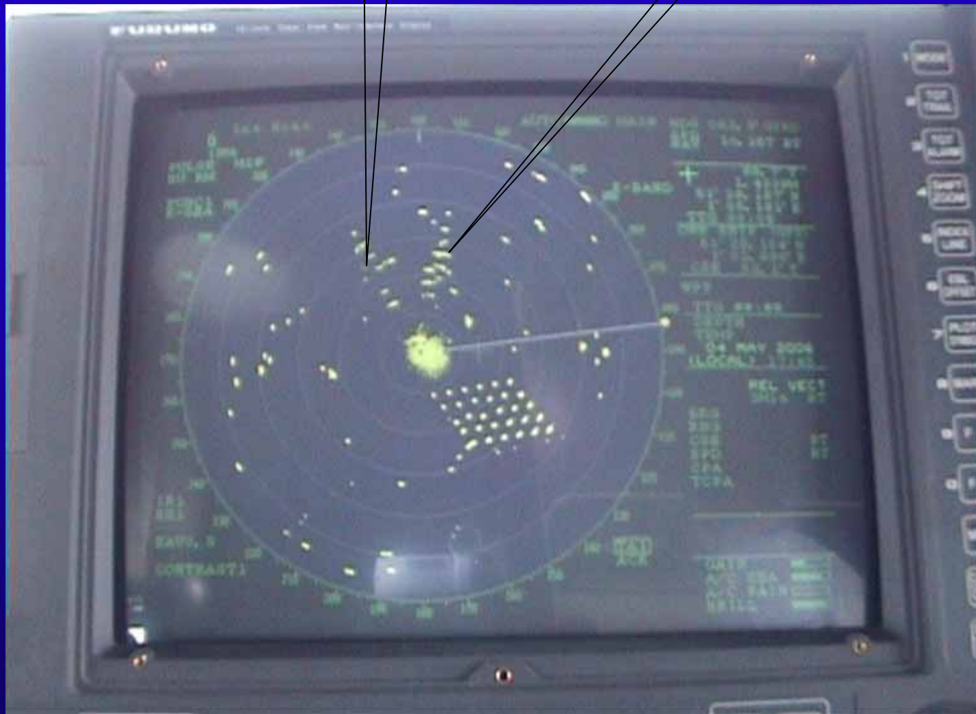
Incomplete external reflected images. Image A is reflected from the Shivering Sands towers and Image B from an overtaking Car carrier
