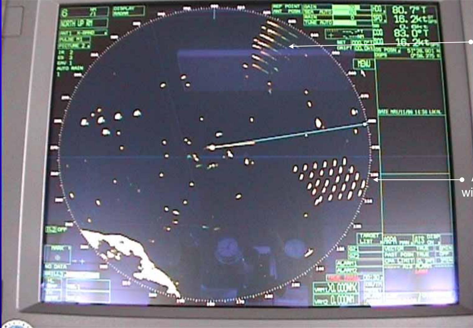
REFLECTIONS; Dredger's radar displayed reflections of wind farm caused by approaching vessel on port bow. The reflections rotated in line as the vessel passed
