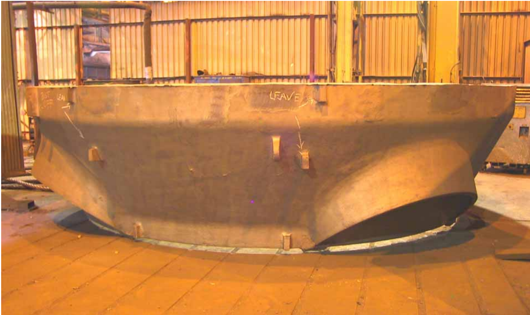
Cast Steel Ring Node 5.5m dia
