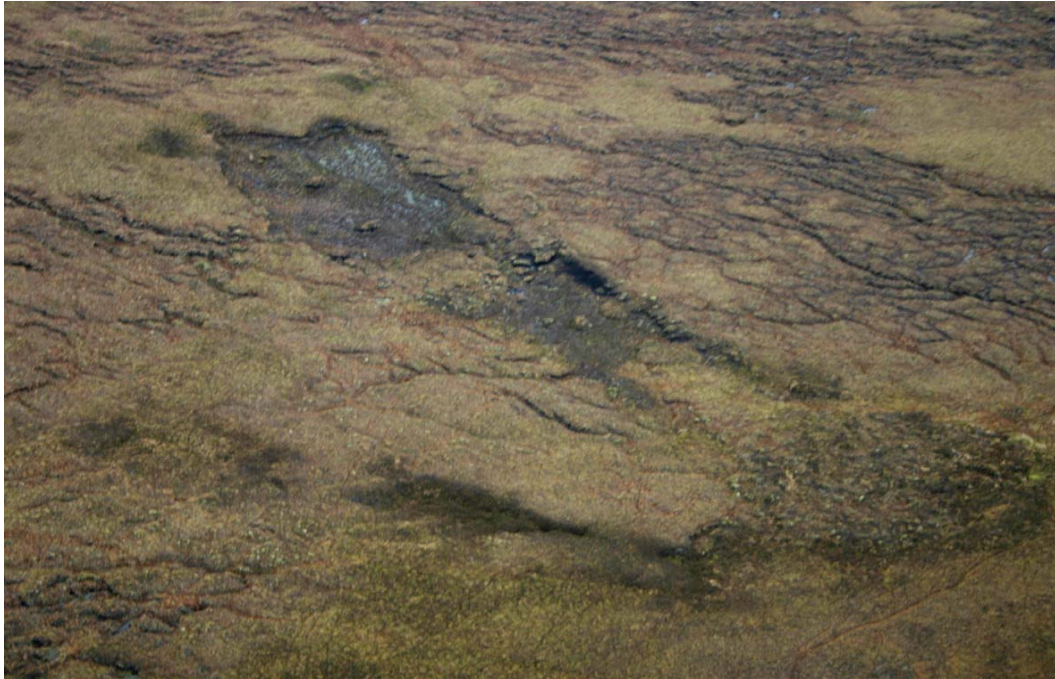
Fig. 4. Major peat slide on hillside showing head, track and run-out zones.
